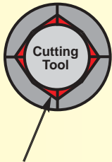
The competition's "Red Zone" . . . A 7mm collet holding a 1/4" cutting tool!
